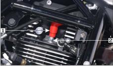
(1) Noise suppressor cap (2) Spark plug
