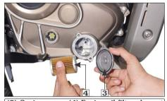
(3) O-ring (4) Engine oil filter element
