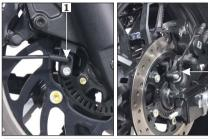
(1) Wheel speed sensor (Front wheel)
