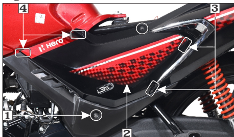
(1) Left side cover screws (2) Side cover (3) Tab/slot (4) Lugs/grommets
