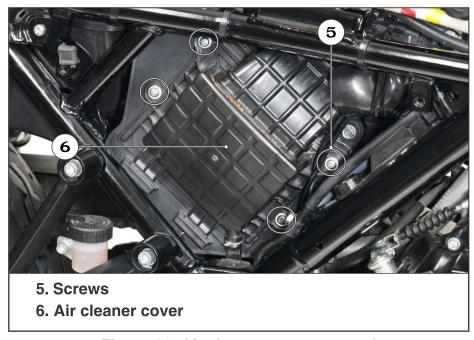
Figure 63. Air cleaner cover removal
