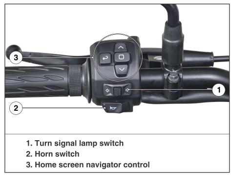
Figure 40. Left handlebar controls
