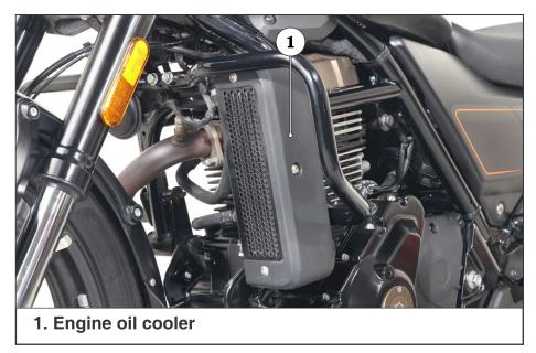
Figure 60. Engine oil cooler
