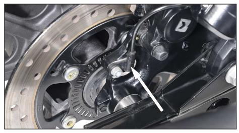
Figure 10. Rear Wheel Speed Sensor (ABS identification)
