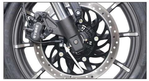
Figure 9. Front Wheel Speed Sensor (ABS identification)
