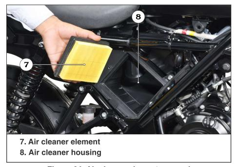
Figure 64. Air cleaner element removal
