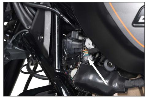
Figure 11. ABS Module (HECU) (located below Fuel tank)
