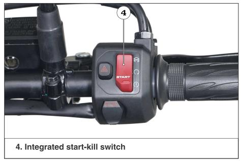
Figure 49. Integrated start-kill switch
