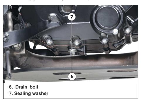
Figure 57. Engine oil replacement
