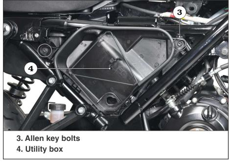
Figure 62. Utility box removal
