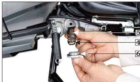
(4) Spring (5) Oil strainer screen (6) O-ring
