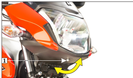
(1) Headlamp adjusting bolt
