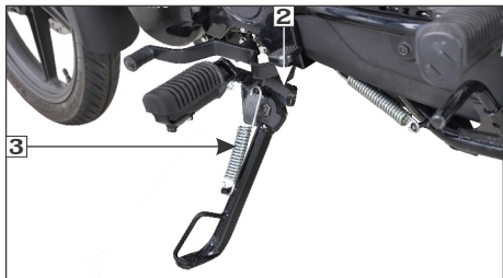
(2) Side stand switch (3) Side stand spring
