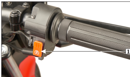
(1) Electric starter switch
