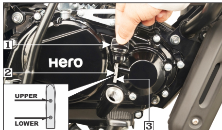
(1) Oil level dipstick (2) Upper level mark (3) Lower level mark
