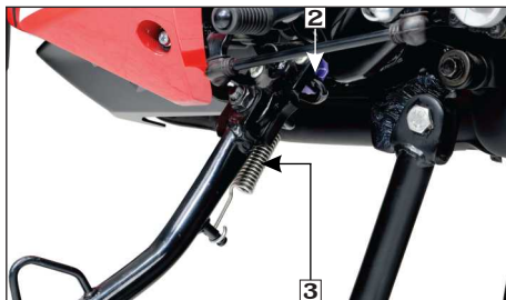
(2) Side stand switch (3) Side stand spring
