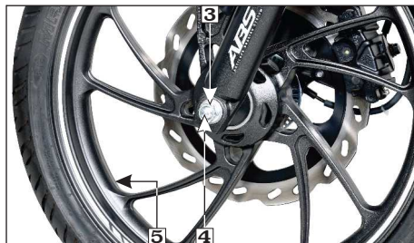
(3) Axle nut (4) Axle (5) Wheel
