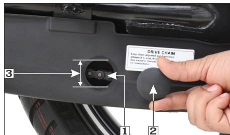
(1) Drive chain (2) Hole cap (3) Drive chain slack: 30 mm
