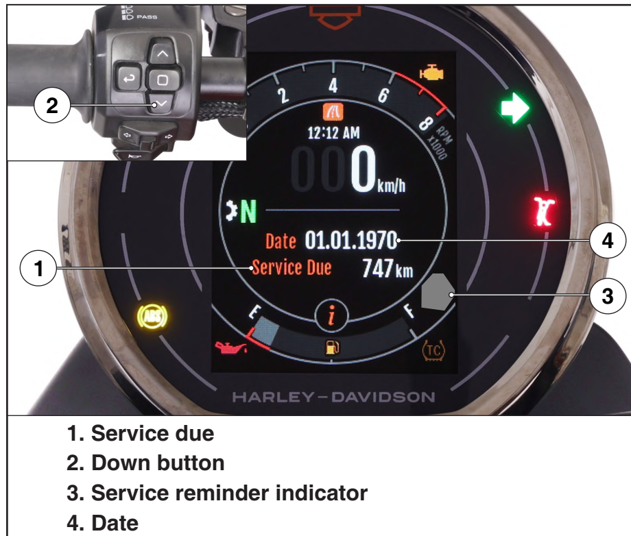
Figure 18. Service due/ Service reminder indicator/Date
