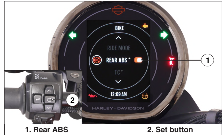
Figure 34. Rear ABS setting
