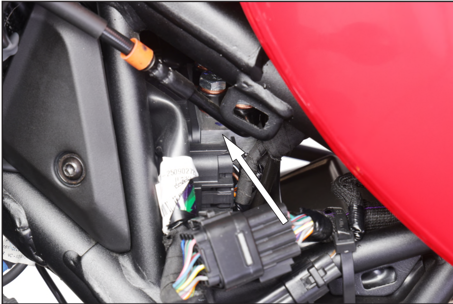
Figure 11. ABS Module (HECU) (located below Fuel tank)
