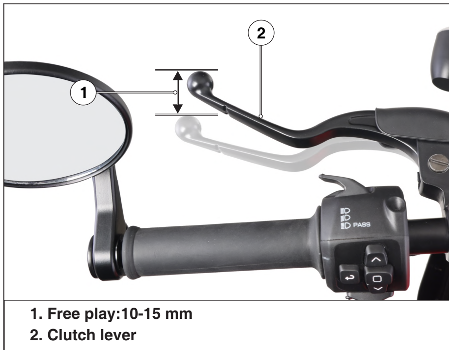
Figure 71. Clutch lever free play
