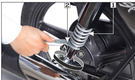
(1) Rear shock absorber adjustment tool (Pin spanner) (2) Pin spanner (A) Stiffer (B) Softer
