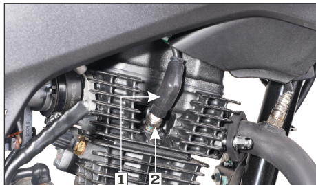
(1) Noise suppressor cap (2) Spark plug
