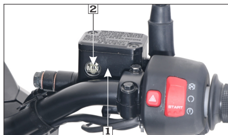
(1) Master cylinder (2) "MIN" mark
