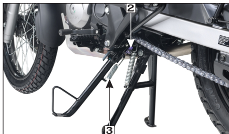
(2) Side stand switch (3) Side stand spring
