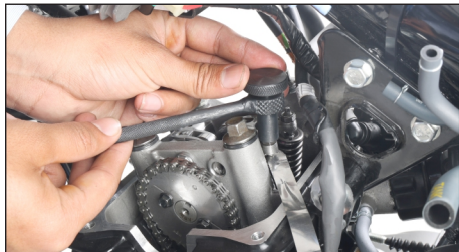
(5) Feeler gauge (6) Adjusting screw (7) Valve stem (8) Lock nut
