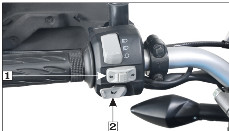
(1) Turn signal switch
