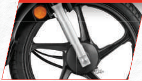
TELESCOPIC FRONT SUSPENSION
